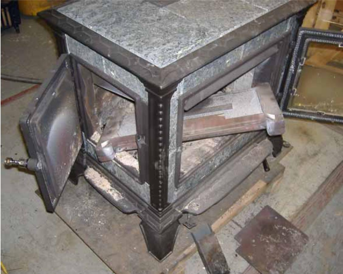
**Photo #1:** The secondary air manifold shown angled for removal through the front door. The side plate and riser are removed to increase the room in the firebox to make this possible.
