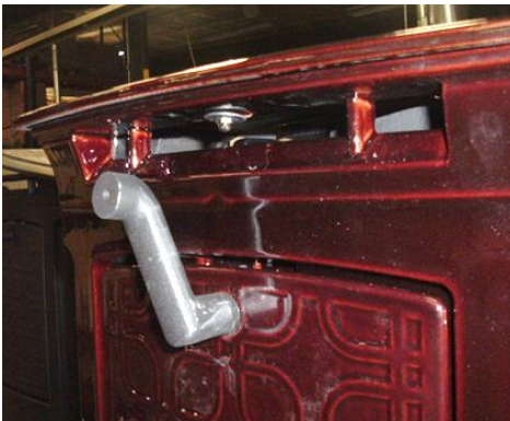
Photo #1: Acorn nut holding the top to the side panel.
