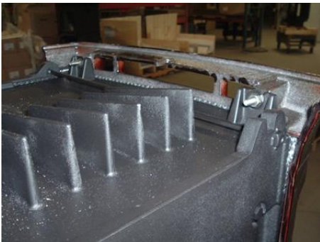
Photo # 2: Nuts and threaded rod holding the top to the side
