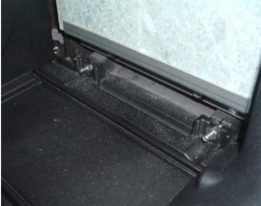
Photo #3: The bottom retaining studs and nuts on the side panel.
