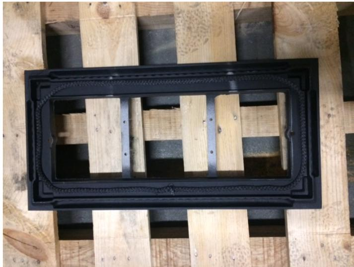
Top Casting rope gasket detail
