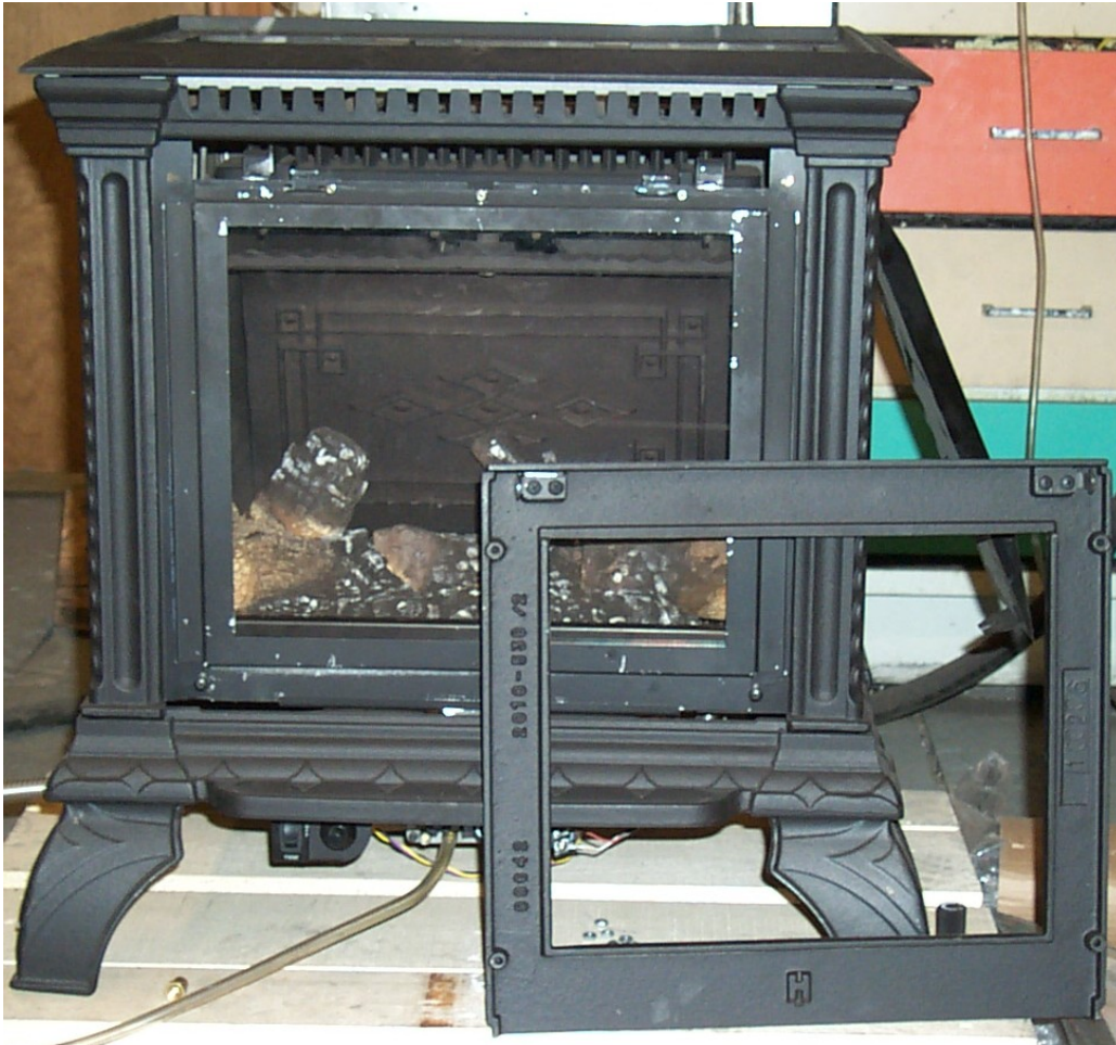
Photo 1 Front removed from stove.
