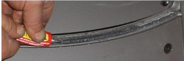
Figure 3: Apply Gasket Adhesive
