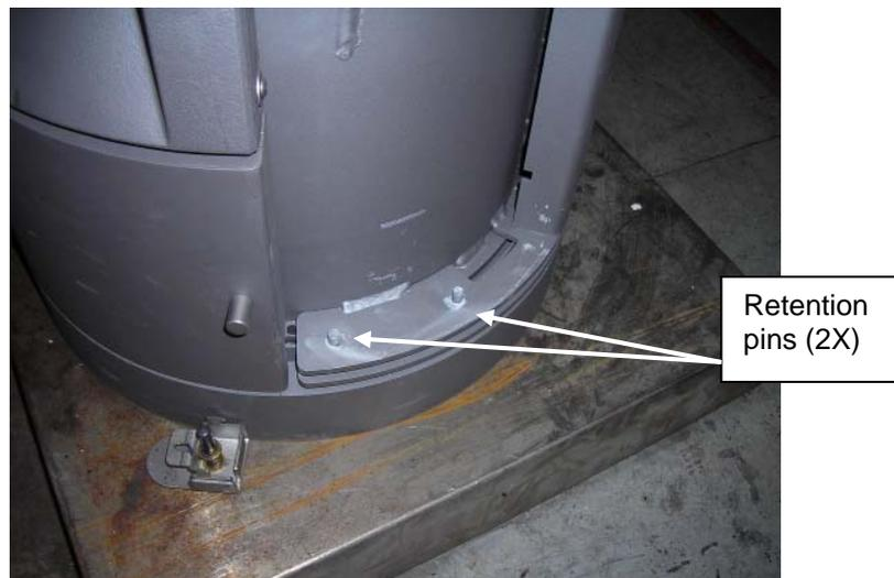
**Figure 1: Bottom stone retention pins**
