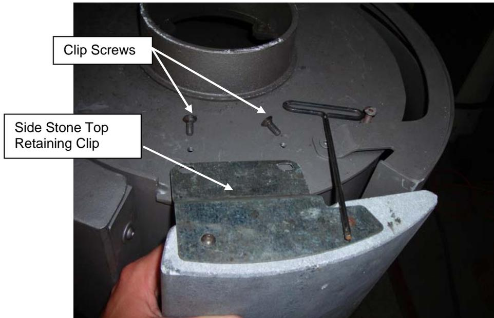
**Figure 2: Securing the Side Stone Top Clips**
