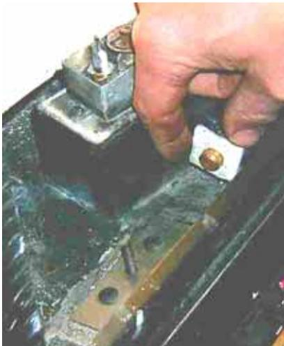
**Photo #11** - Place the white ceramic Gasket over the burner orifice.
