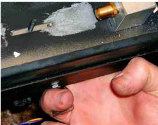
**Photo #5** – Lower plate held under the firebox
