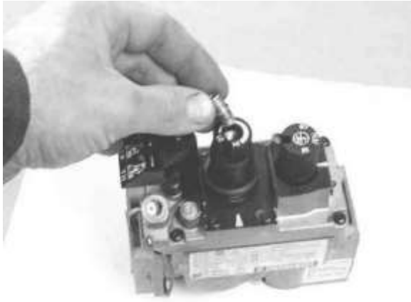
Figure 5 – Conversion Plug, Removed
