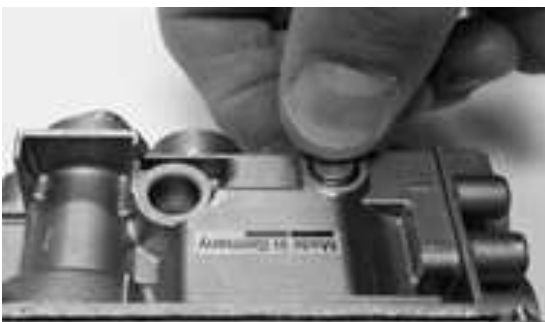
Figure 15 – NG Low Pressure Screw Insertion
