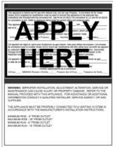
Figure 18 – Rating Plate Conversion Label Location
