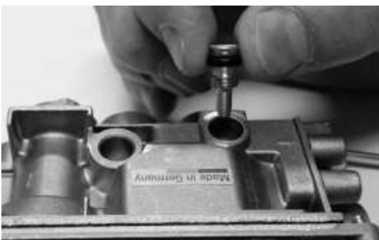
Figure 15 – NG Low Pressure Screw Insertion
