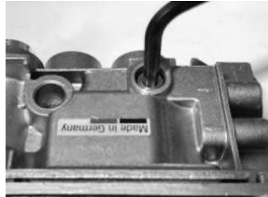
Figure 17 – Tighten NG Low Pressure Orifice
