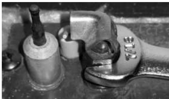
Figure 2 – Loosening Pilot Tower
