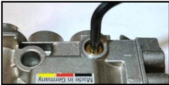
Figure 8 – Adjusting Low Pressure Orifice
