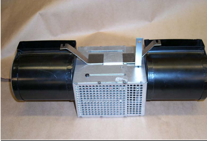
Photo #2 – Hanger mount slots are positioned for the Tucson or Stowe (slots forward) and L-Bracket is installed for the Tucson (screwed to forward hole- rear hole can be seen behind the L-Bracket). Blower housing is compressed for the Tucson & Stowe models.
