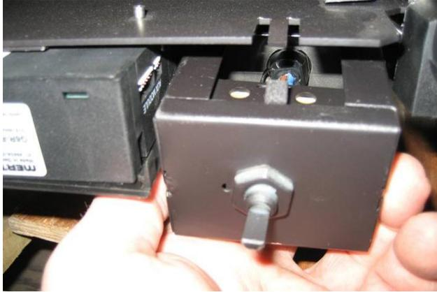
Photo #7 – Slide Rheostat Housing onto Tab
