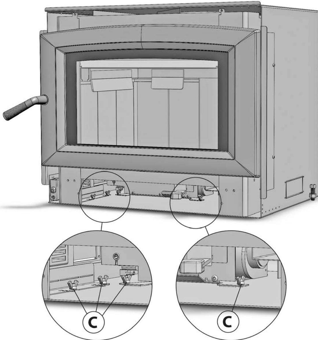
4. Carefully pull the blower assembly towards you to remove it from the convection air jacket. Disconnect the wires from the faulty blower once they are accessible. Replace the faulty blower with the new blower and reconnect the wires to the same points from which they were removed.
