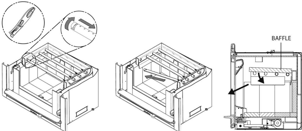
**Install the new baffle:**
